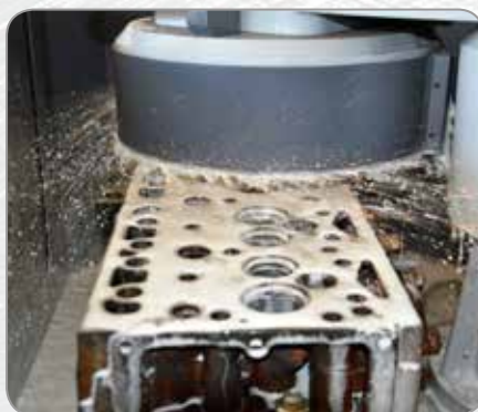
WET SURFACE GRINDING WITH COOLANT FLUID
